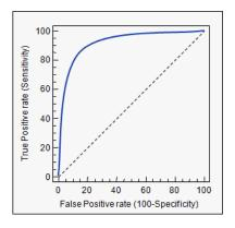
Given a confusion matrix, a ROC curve is a plot of the False Positive Rate (FPR) on the x-axis and the True Positive Rate (TPR) on the y-axis.
